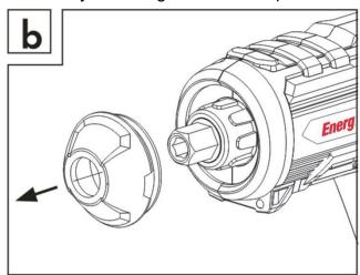
• Now you can fit the supplied attachments to the appliance in 45°steps. Fit the attachment onto the appliance so that the attachment clicks into place. (See fig. C, example: torque attachment).
